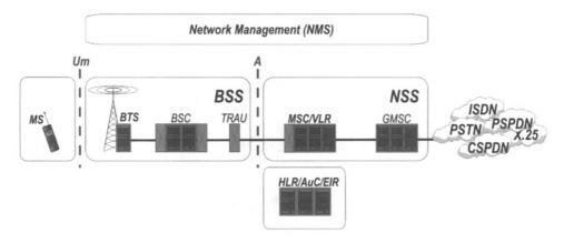
Figure 2.2. Basic GSM network and its subsystems
