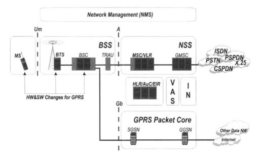
Figure 2.6. General packet radio service (GPRS)
