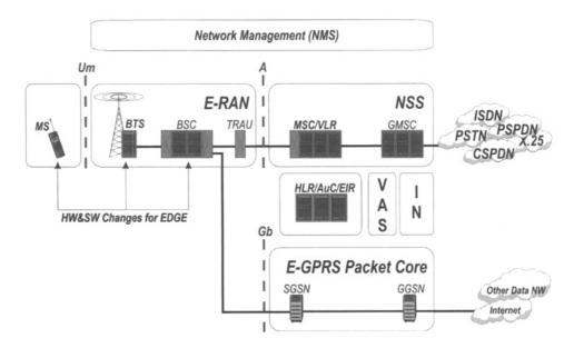
Figure 2.7. Enhanced data rates for global evolution
