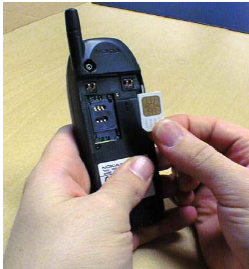
Figure 3. Inserting a SIM card in a mobile phone
