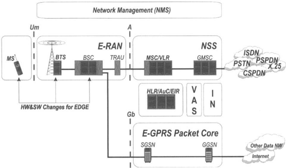
**Figure 2.7.** Enhanced data rates for global evolution
